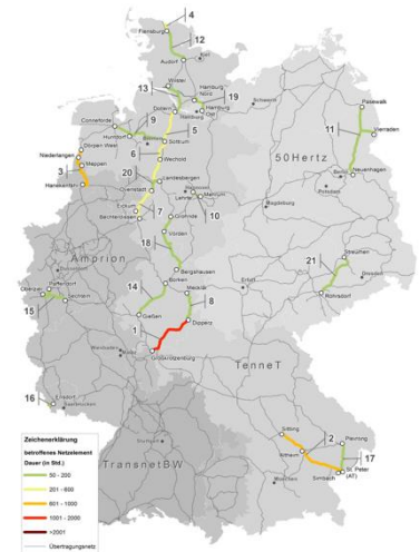
Duration of congestion measures on the most affected lines in Germany in 2019 (from the Bundesnetzagentur's monitoring report)
